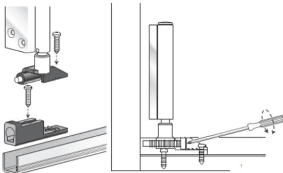
\* Pre drill hole for pivot block, apply sealant before fastening screw.
