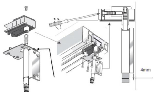
Top Pivot Block is installed in one piece
