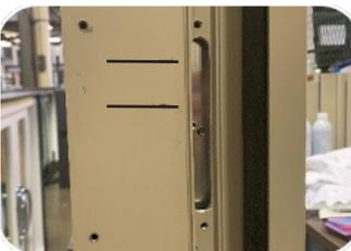
**REMOVE THE PLATE AND PRE-DRILL THE MARKED HOLES WITH A 9/64 BIT.**
